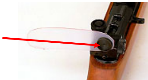
A rear sight blinder can be made from a piece of translucent plastic. Cut a hole in one end so that the blinder will fit over the detached rear sight iris
